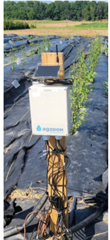
Figure 1. An Ag-Zoom data logger/control unit monitoring and controlling irrigation for tulsi-basil at WyeREC.
