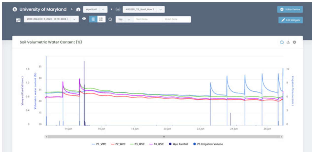
Figure 2. The dashboard interface of Ag-Zoom. Soil Volumetric Water Content (VWC) measured by four capacitance sensors is depicted by different color horizontal lines. Rainfall and irrigation events with volumes are represented by vertical lines (different colors). Each irrigation event increases soil volumetric water content as depicted by the peaks in VWC. Drainage through the soil profile in the raised bed indicates soil moisture at capacity.
