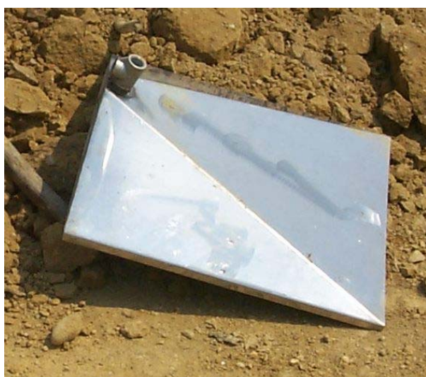
Figure 2. A pan lysimeter before it was placed in a trench.
