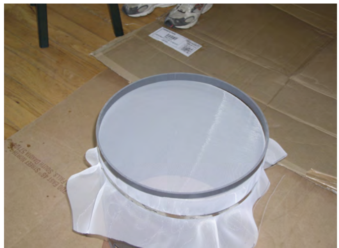
Figure 13. Rings must be softened in the oven to stretch them onto the silos.
