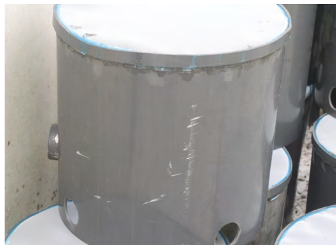
Figure 17. The excess mesh is trimmed and the hose clamp is removed.
