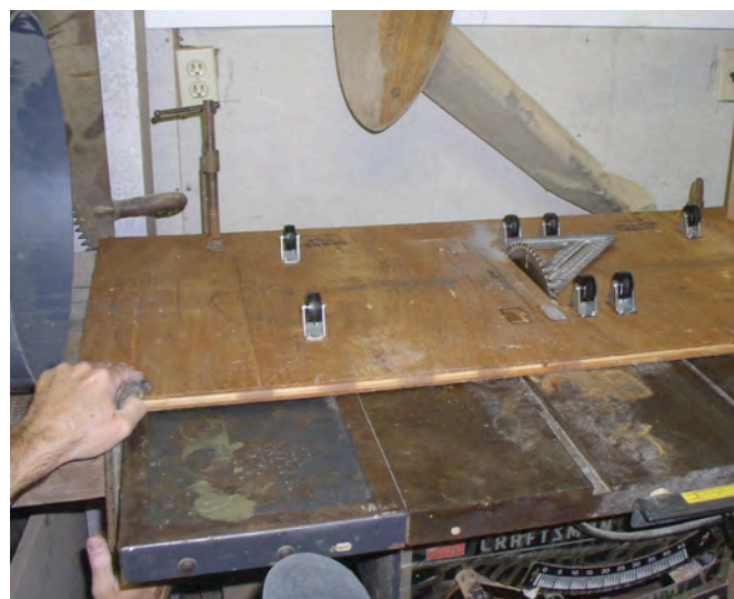
Figure 3. A simple jig to assist in cutting silo sections clamped to a table saw.
