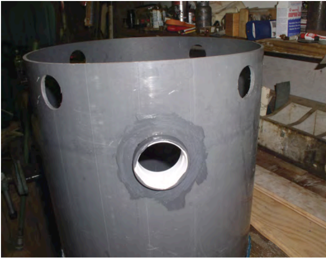
Figure 18. The connector is glued in place.
