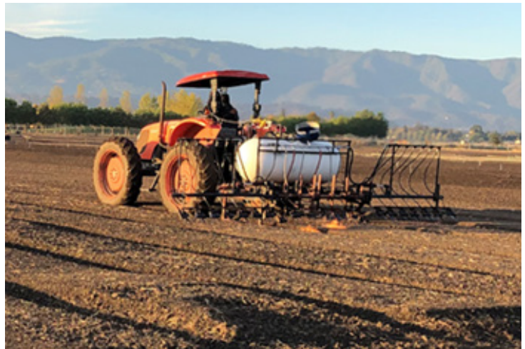
Fig. 1. Tractor equipped with propane tank and burners. Attribute: Ian Abbott (CC)
